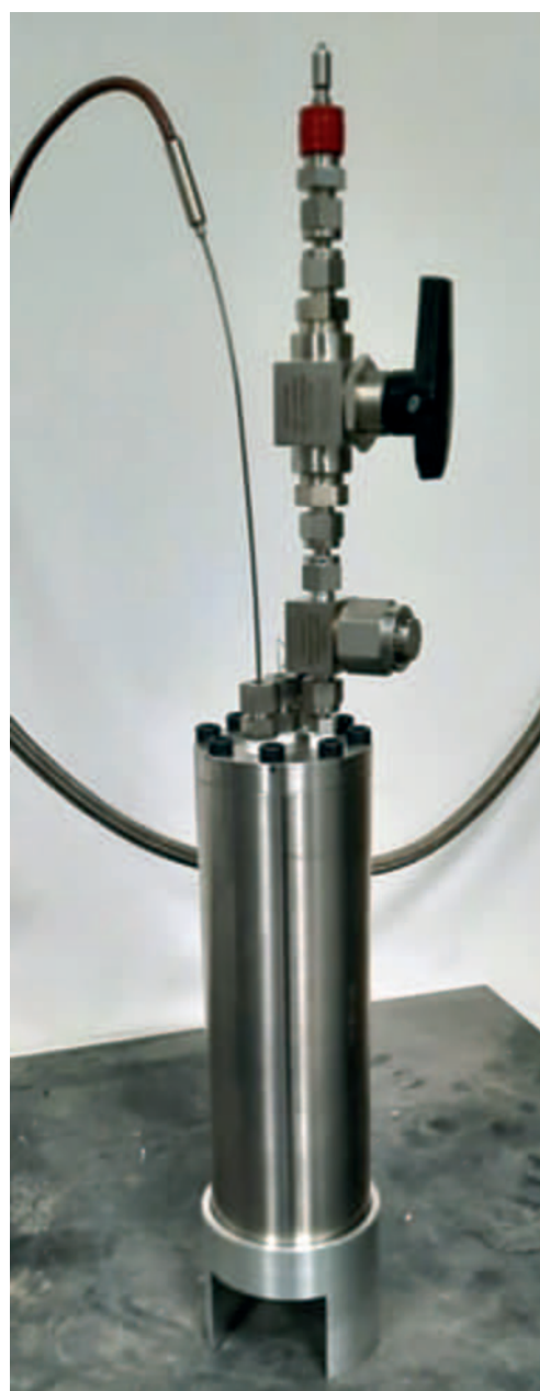
Figure 8: Test tank assembled at MAHYTEC to carry out thermal conductivity tests with the selected method, MAHYTEC designed the test tank with FHa support, which takes care of the assembly of the test bench in parallel.
