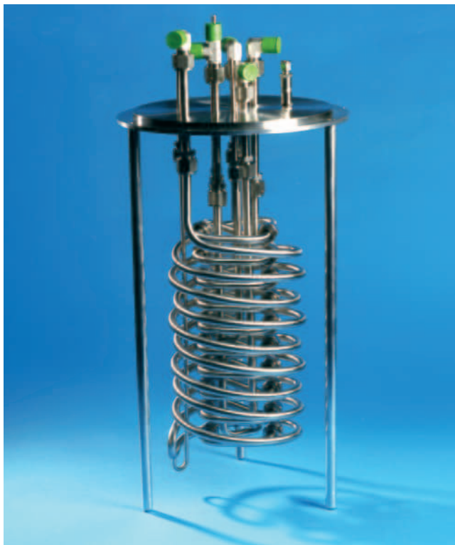
Figure 2: Saturator component of an NPL-designed dew- and frost-point primary generator
