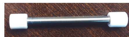
Figure 2: Example of sorbents for VOCs sampling/enrichment
