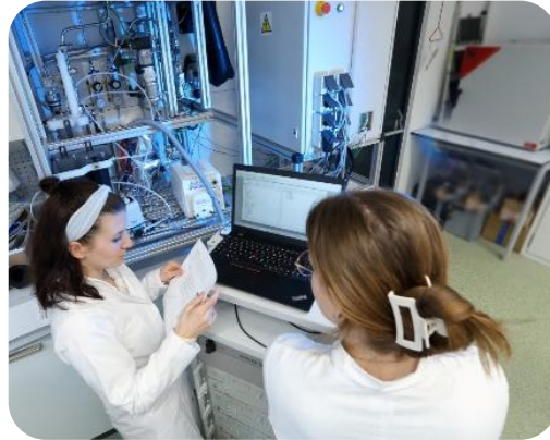
PEM Single Cell Test Bench
